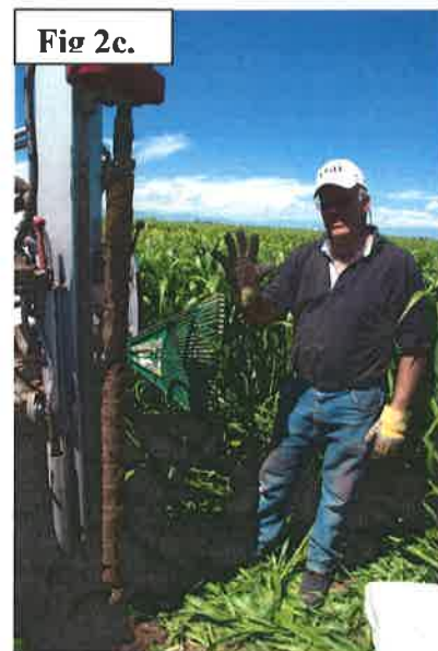
Figure 2. A Giddings truck mount was used for collection of soil samples to assess the potential for cover crops to scavenge, recover and cycle soil nitrogen (nitrate-nitrogen, \text{NO}_3\text{-N} ) and other nutrients. The truck is set up in the middle of the plot after the cover crop aboveground sample have been collected (Fig. 2a), the probe is inserted to 5 feet (Fig 2b) and the soil sample is separated in bags and put in coolers for laboratory analysis (Fig 2c).
