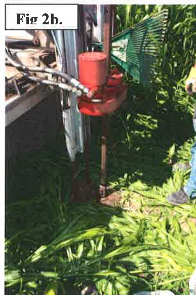
Figure 2. A Giddings truck mount was used for collection of soil samples to assess the potential for cover crops to scavenge, recover and cycle soil nitrogen (nitrate-nitrogen, \text{NO}_3\text{-N} ) and other nutrients. The truck is set up in the middle of the plot after the cover crop aboveground sample have been collected (Fig. 2a), the probe is inserted to 5 feet (Fig 2b) and the soil sample is separated in bags and put in coolers for laboratory analysis (Fig 2c).
