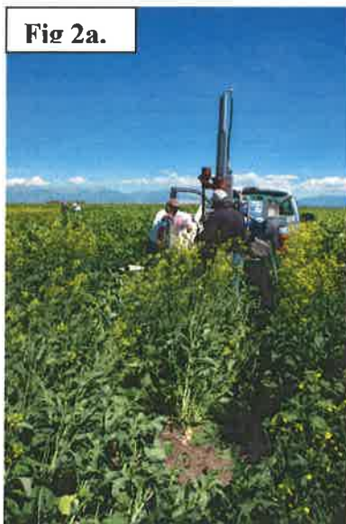
Figure 2. A Giddings truck mount was used for collection of soil samples to assess the potential for cover crops to scavenge, recover and cycle soil nitrogen (nitrate-nitrogen, \text{NO}_3\text{-N} ) and other nutrients. The truck is set up in the middle of the plot after the cover crop aboveground sample have been collected (Fig. 2a), the probe is inserted to 5 feet (Fig 2b) and the soil sample is separated in bags and put in coolers for laboratory analysis (Fig 2c).
